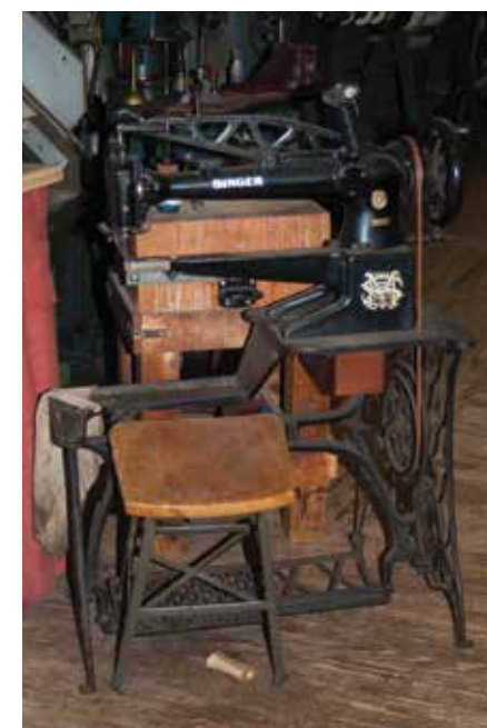
It takes skillful hands, 125 steps and 17 machines to make a pair of boots. Machines from founder A.M. Kroop's day include the shop's oldest, a 1916 Singer. In addition to the wall of boot lasts, there is a wall of dies to cut the leather.
